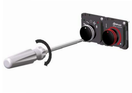
Fig. 17 - Secure Control Panel
