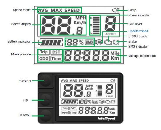
**ON/OFF** - Press and hold Power button for 1.5 second can turn on/off the display. The Display can automatically shut down when there is no operate & ride for X minutes (X could be  $0 \sim 9$ ).
