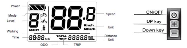
**ON/OFF** - Long press On/Off to start display. Long press On/Off again to switch off. Display off automatically after no any operation on vehicle for ten minutes (default).
