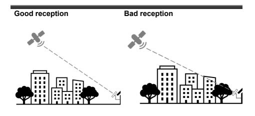
Obstacles like tall buildings, bridges, trees, heavy rain, snow, ice, and cloud can block this view and can cause a loss of signal/picture.
